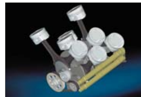
■ The piston arrangement of the Volkswagen W8.
