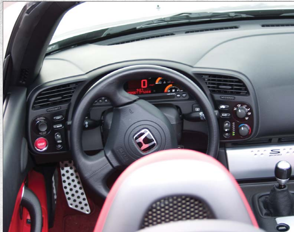
The instruments and controls on the S2000 are remarkably clean, simple and yet remarkably thorough, from audio controls to the left and HVAC to the right of the wheel, to the digital tach.
