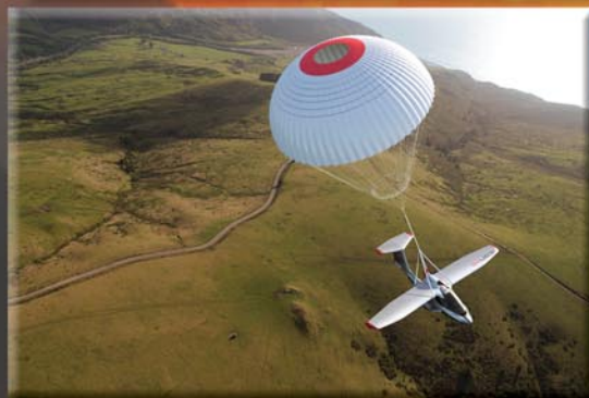
An optional ICON Complete Airplane Parachute brings the entire airplane gently to the ground in case of an emergency.
