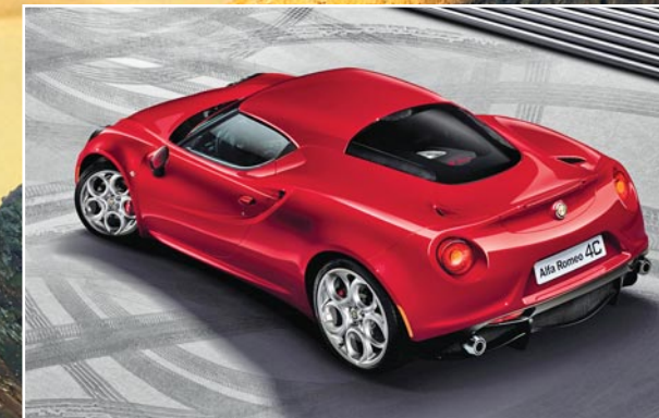
2015 Alfa Romeo 4C has a 240-hp 1.7L four, 6-speed automated manual transmission and rear-wheel drive. Estimates are around $60,000.
